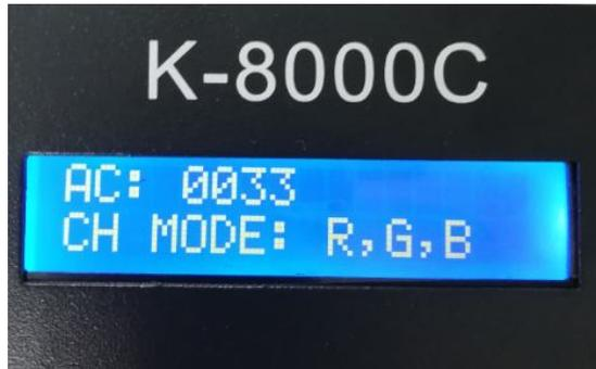
6. Press the “MODE” button again to enter the “MC” manual test mode. “Speed+” and “Speed-” can adjust the pixel points (long press “Speed+” or “Speed-” to quickly increase or decrease), the lamps are brightened one by one; The controller displays as shown below
