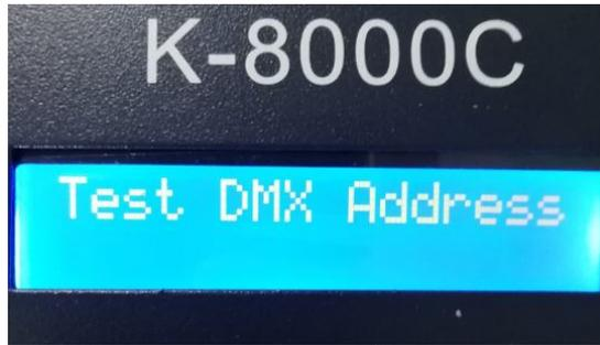
2. It takes about 2 seconds to enter the lights address interface, the controller displays as below:
