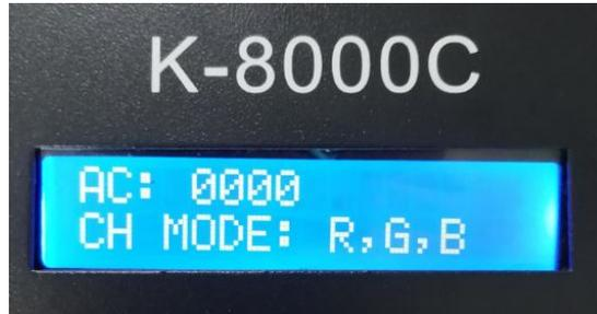
3. Press the “MODE” button to start the test and switch channels selection; Press the “CHIP” button to switch the manual and automatic channel testing mode;
