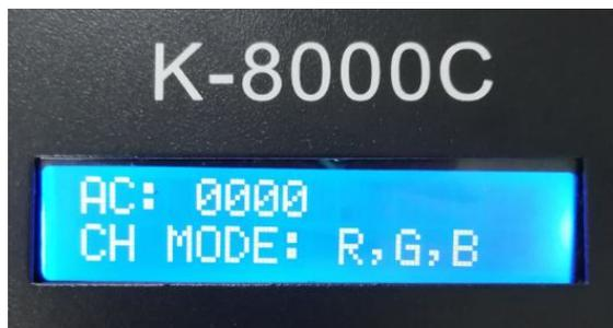
5. Press the “MODE” button to enter the “AC” automatic test mode, the lamps will start to run in sequence; the controller will display the following picture (the interval channel is set to be unadjustable when writing code)
