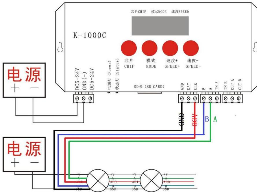
DMX512 single line signal wiring diagram: **A(DAT)/ADD/GND**
