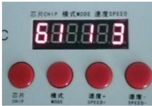
8. Press and hold "Chip CHIP" first, then press the "Mode MODE" button to switch to playback mode and switch the chip to Chip: 10, it is the DMX512 standard protocol 250Kbps playback mode. At this time, press the mode button and the speed button to switch the playback mode and adjust the speed respectively, as shown below:
