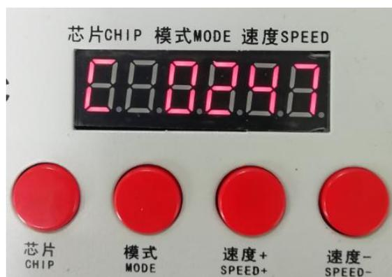
7. After the test is completed, press "CHIP" to exit the channel test and return to the write code interface;
