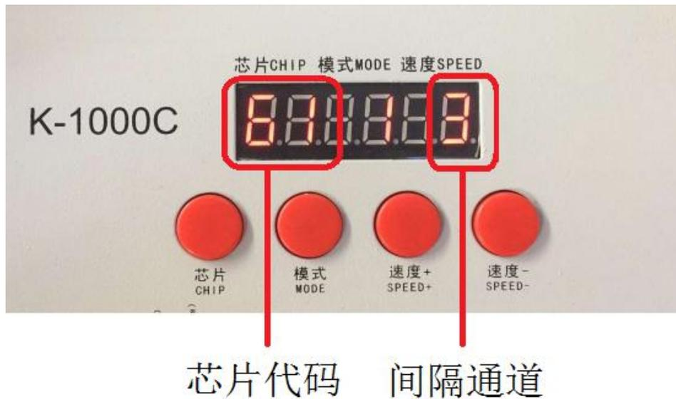
2. Press the "Chip CHIP" button to select the DMX512 onboard IC model; "Speed+" and "Speed-" select the fixture interval channel (0-99).
