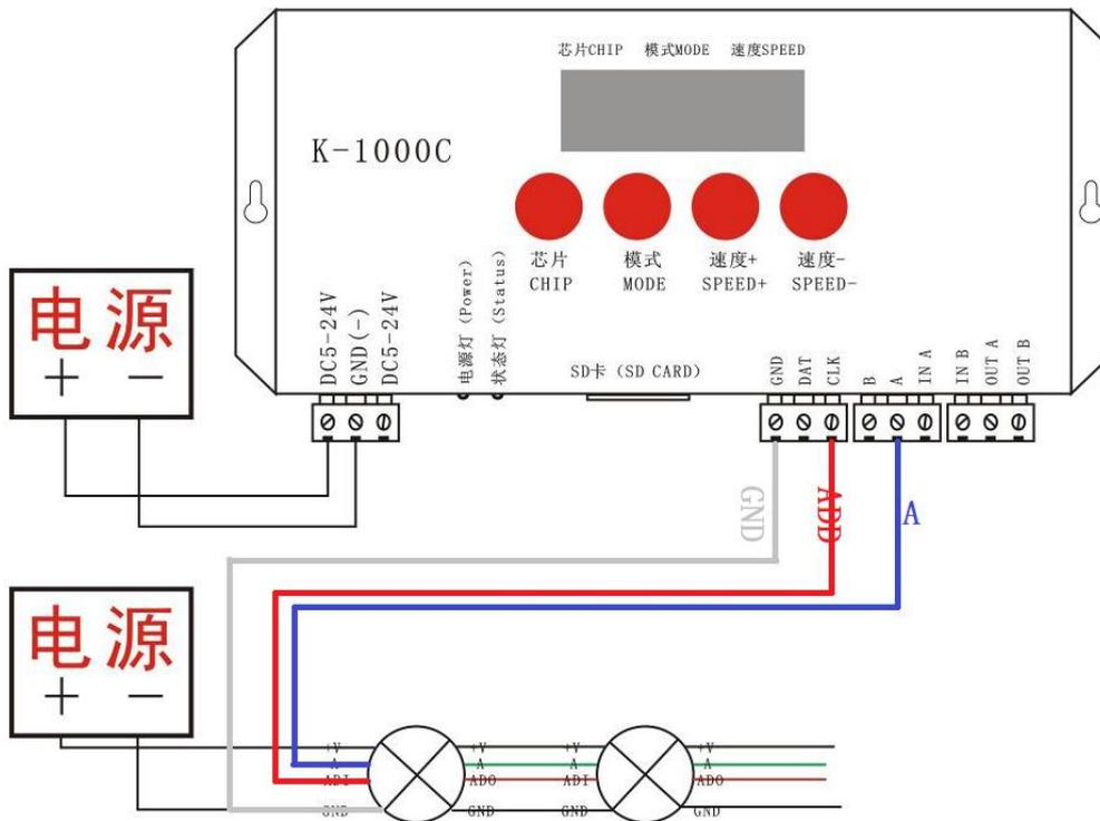
Note: For some DMX512 luminaire installations, the controller output terminal does not need to be connected to the ADDR write address line of the luminaire. It only needs to be connected to A/B/GND, and its data bus is automatically addressed (for details can refer to the DMX512 luminaire loaded IC usage specification).
