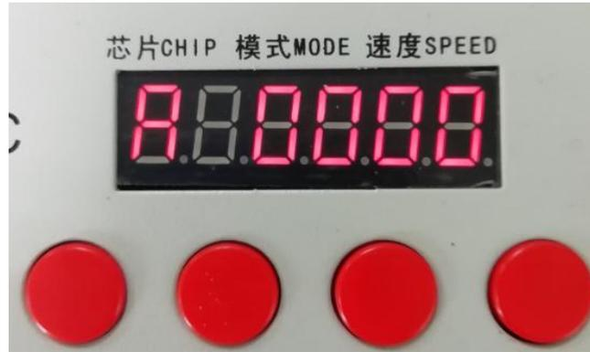
5. Press the “MODE MODE” button to enter the automatic test mode, the display is “A \*\*\*\*” (\* is the number of channels), and the fixture will automatically start the white light from the first pixel.
